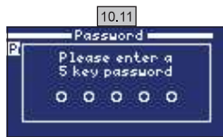
10.11 Password: Protects user access to the menu by activating a password. Press a combination of 5 keys and the system will memorize it. If you forget the password, there is a 'master password'. Ask your installer/supplier.
