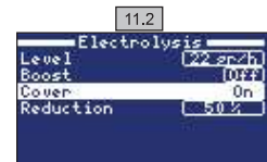
11.2 Reduction of chlorine production (as a percentage), when the pool cover is closed. With the cover closed it is not necessary for the system to run at 100%. Use this parameter to regulate the optimal amount of chlorine produced.
